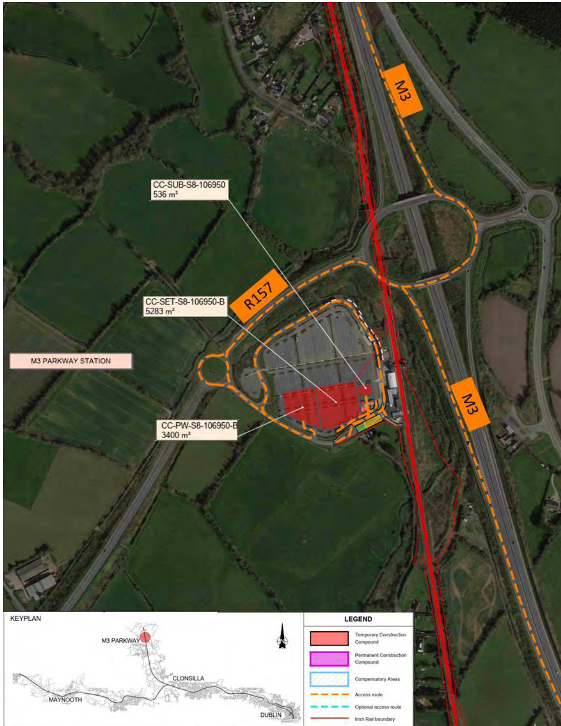
Figure 5-292 M3 Parkway substation compound and haulage route
