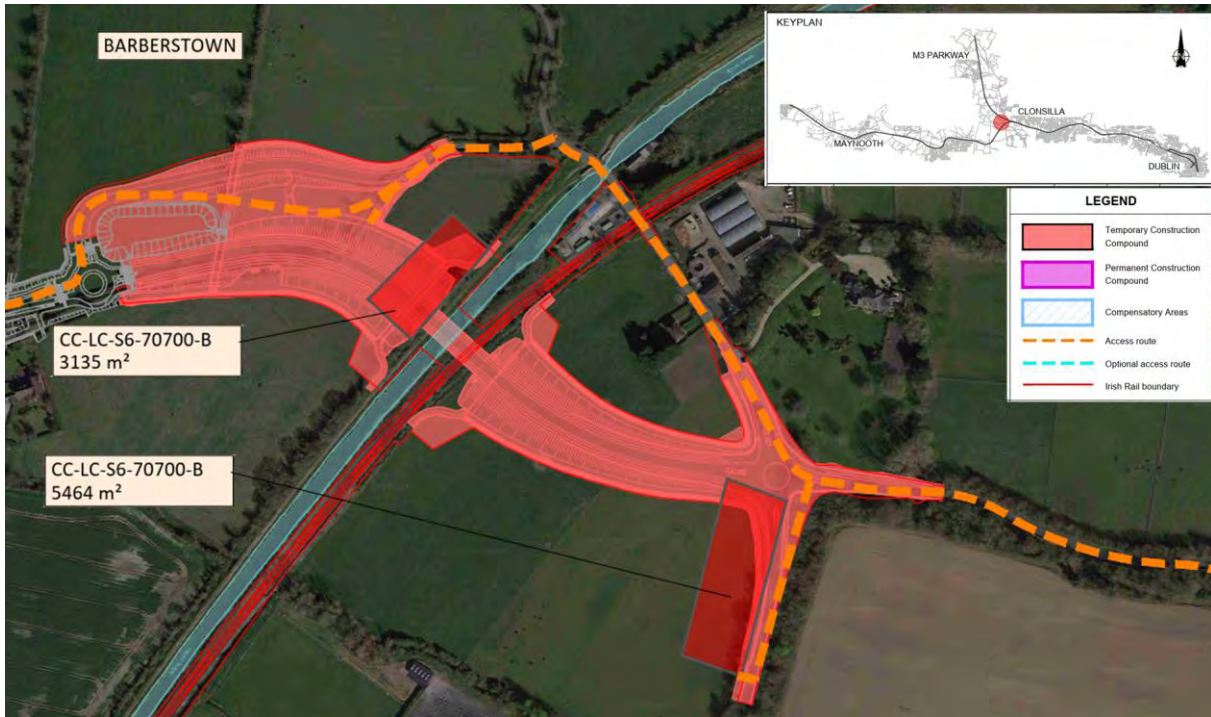
Figure 5-301 Barberstown level crossing compound
