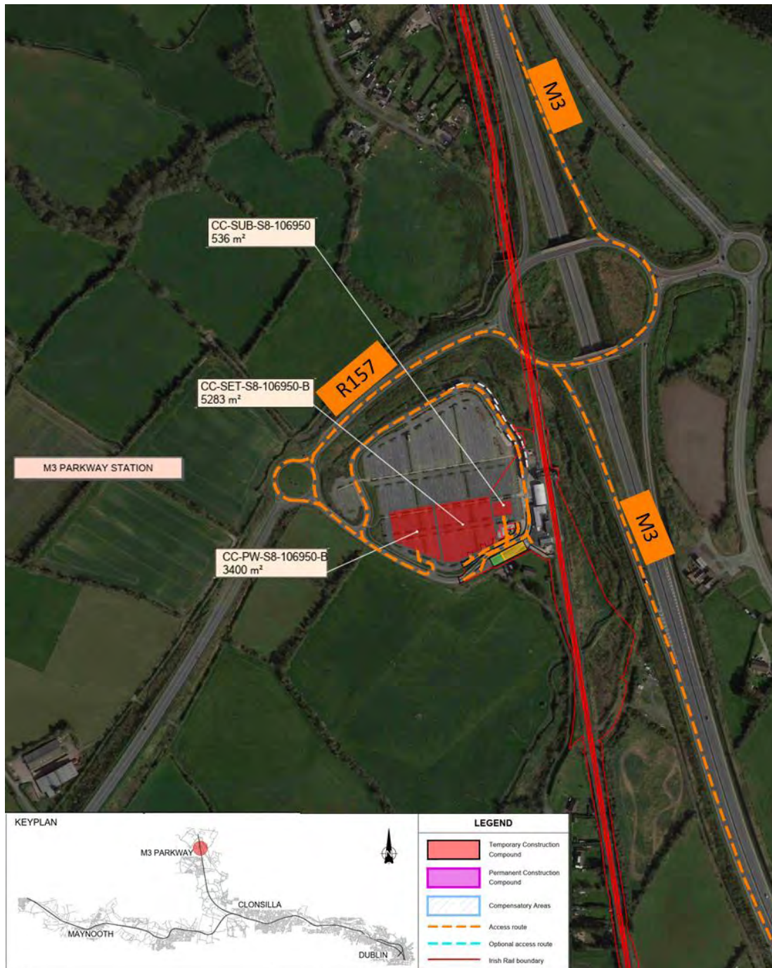
Figure 5-295 M3 Parkway permanent way construction compound and haulage route
