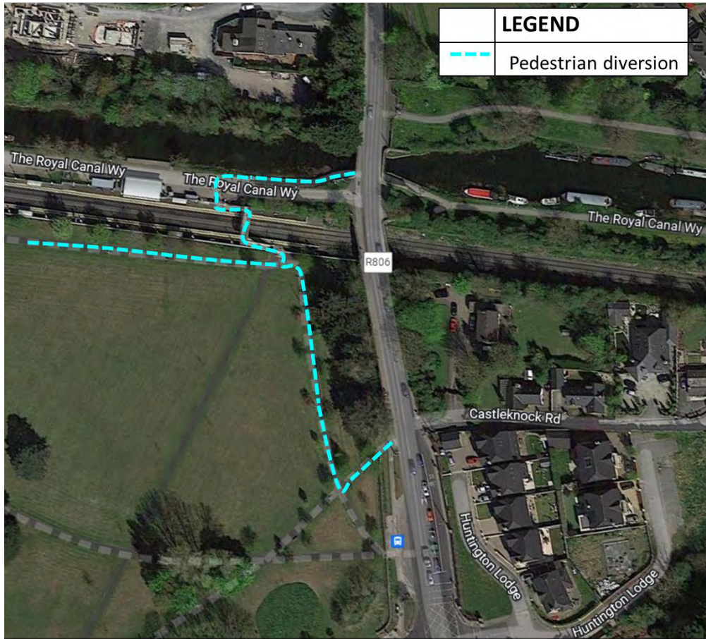
Figure 5-262 Pedestrian diversion during OBG11 construction
