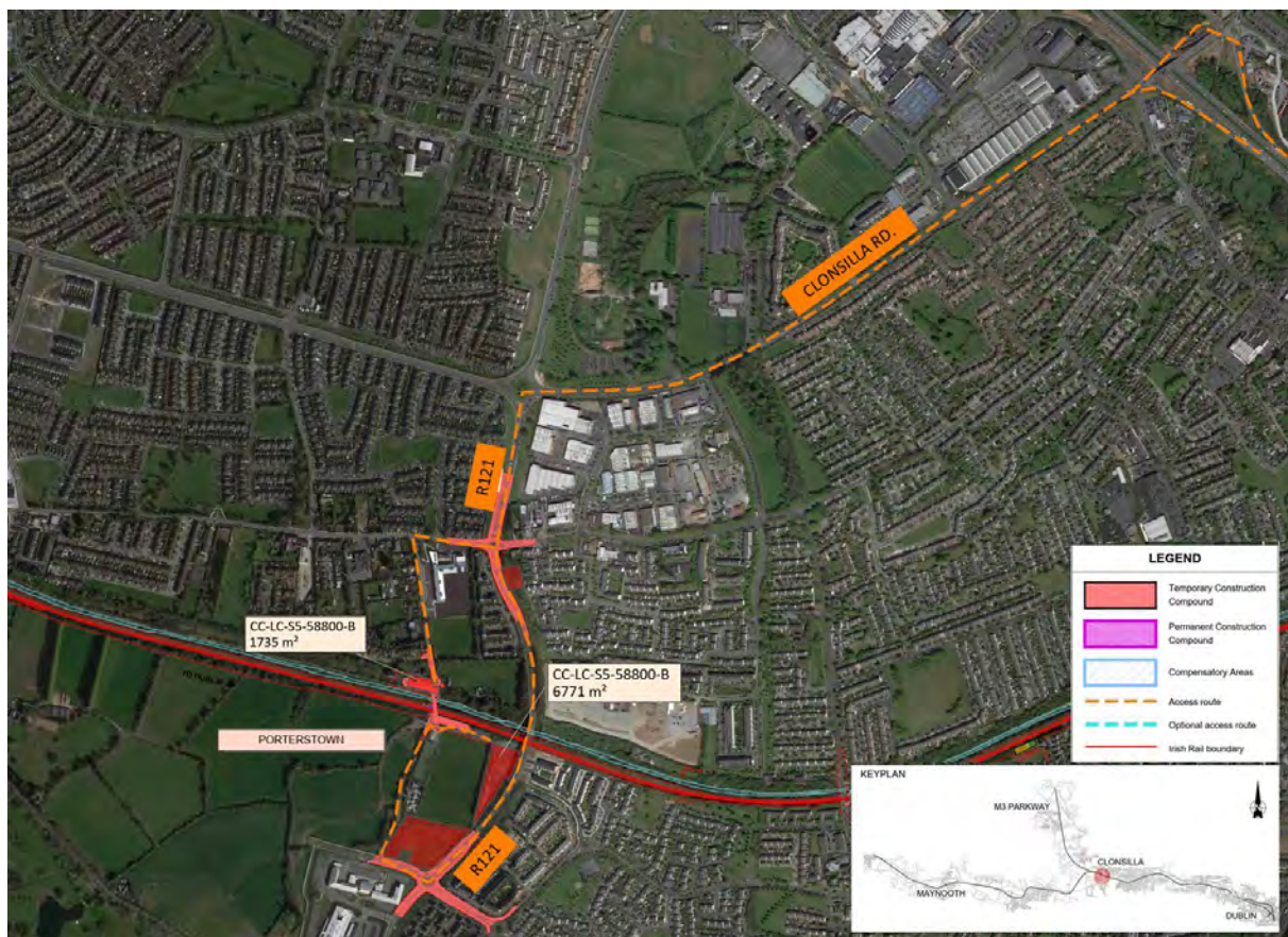
Figure 5-273 Porterstown level crossing compound
