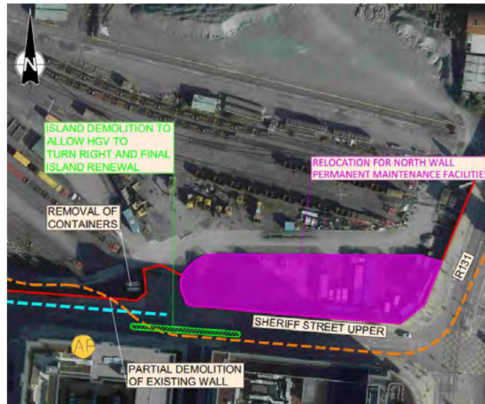
Figure 5-131 Traffic island demolition
