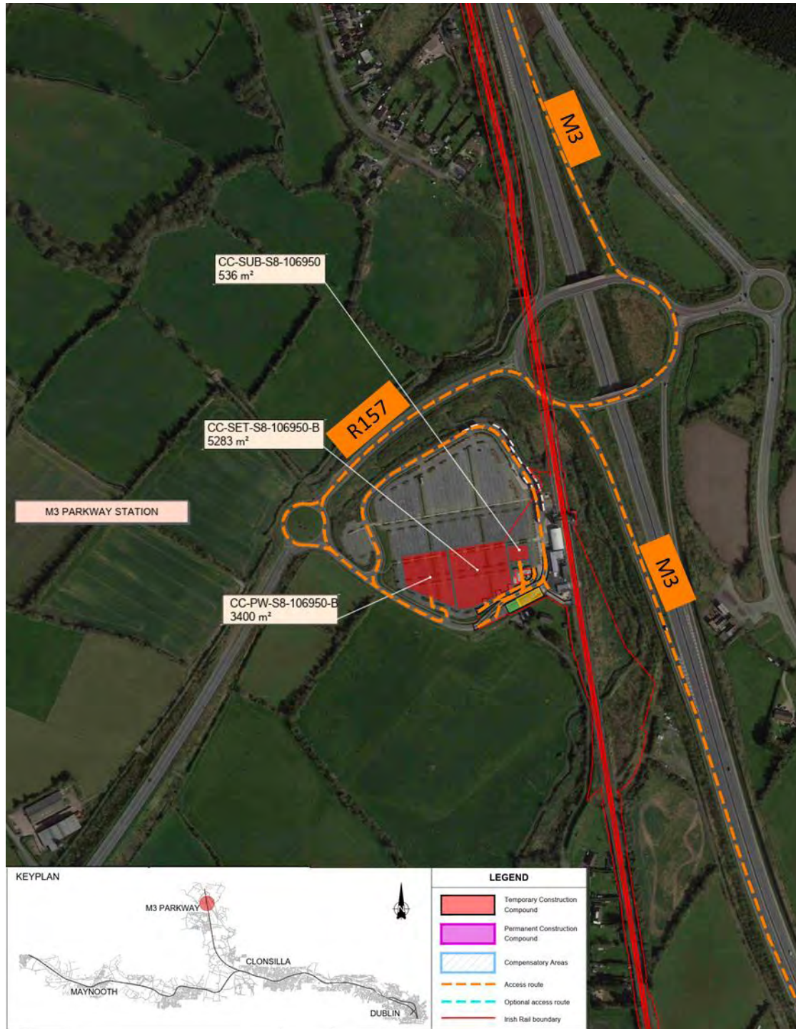
Figure 5-283 M3 Parkway SET compound and haulage route
