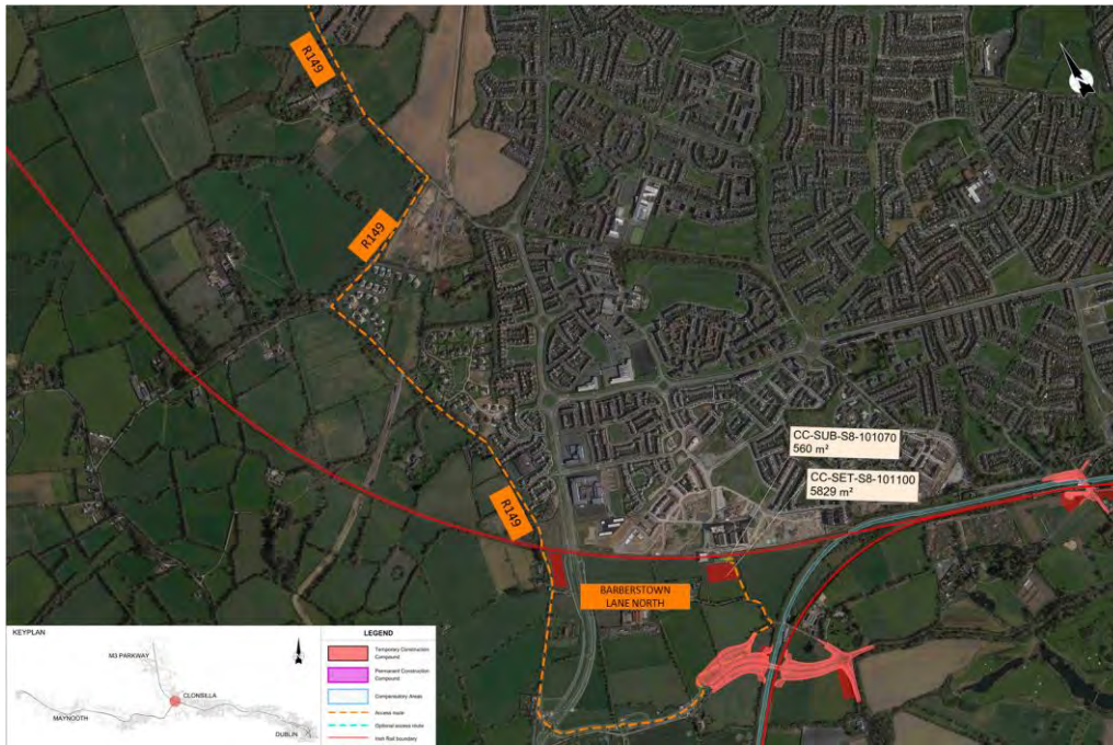
Figure 5-284 Hansfield substation compound and haulage route
