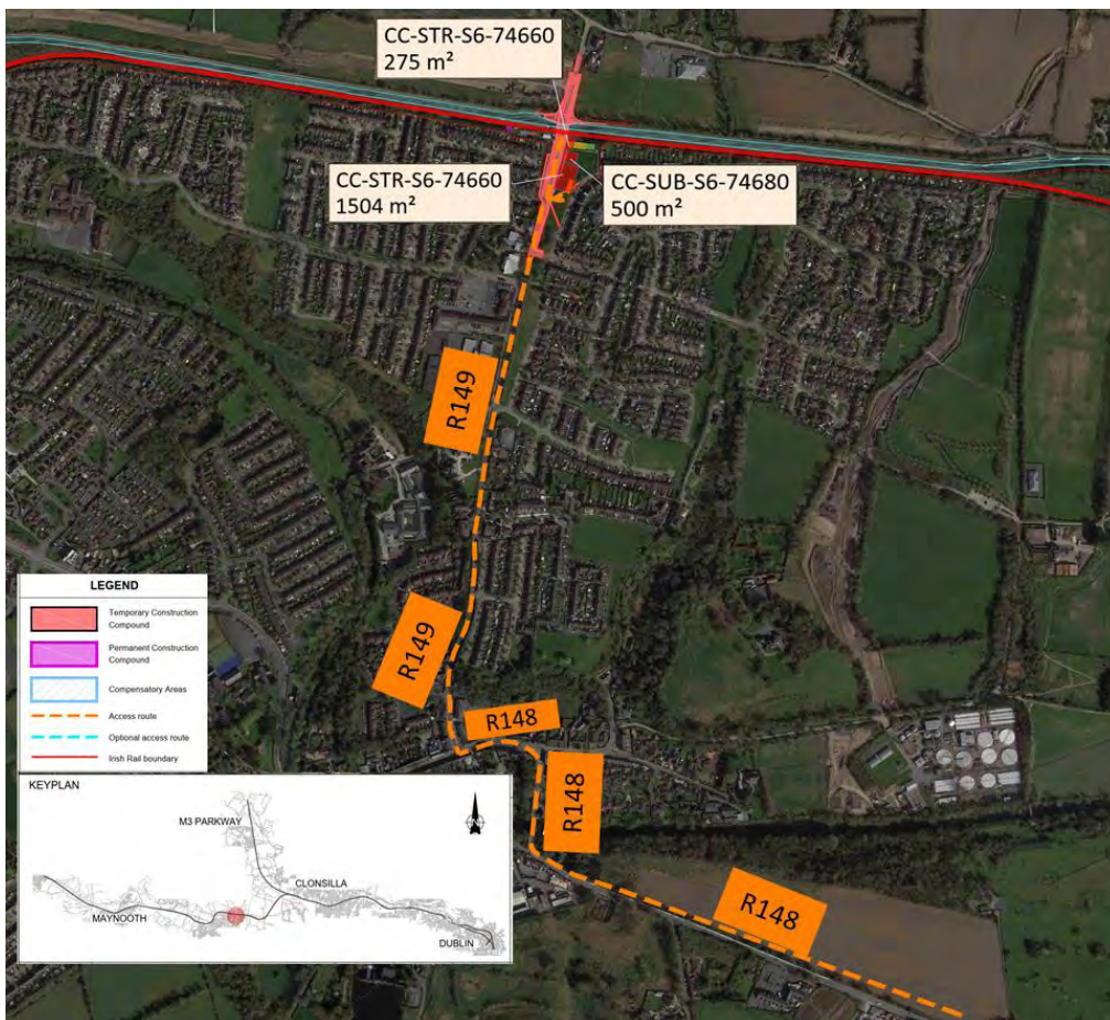
Figure 5-316 Leixlip Confey substation compound and haulage route
