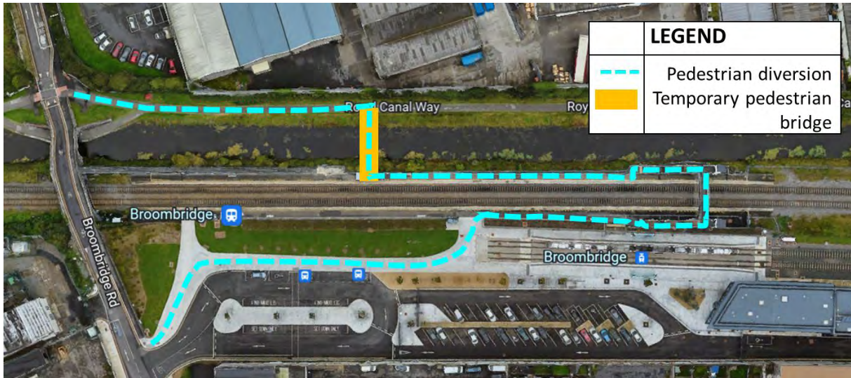
Figure 5-233 Pedestrian diversion via temporary ramp at OBG5
