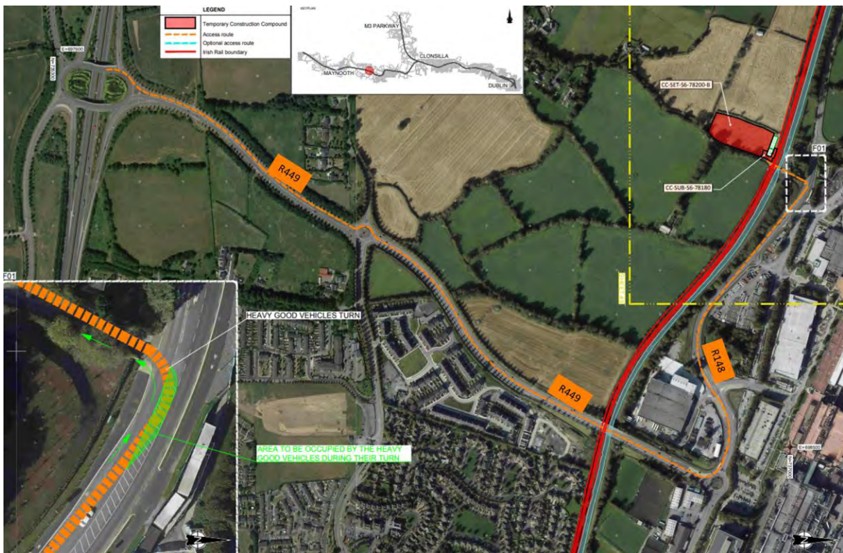
Figure 5-326 Blakestown substation compound and haulage route
